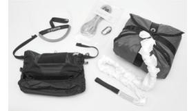
Connect your rescue risers to your parachute with the maillon. Tighten it with pliers. Do not overtighten. ¼ turn past finger tight is ideal.
