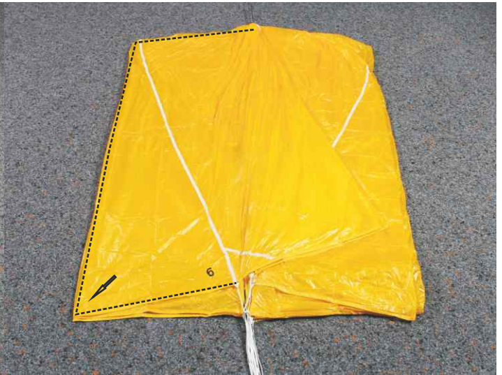
14. Arrange panel 6 (Ultra Cross 100/125). Ultra Cross 150: panels 8,7
