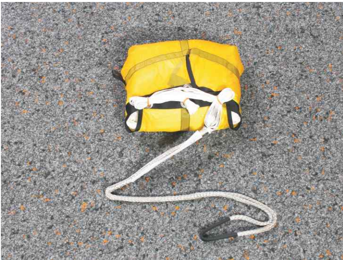
28. Close the deployment bag with the lines. First in the middle then the sides.
