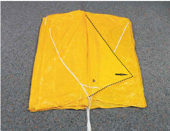
7. Arrange panel 4 (Ultra Cross 100/125). Ultra Cross 150: panel 5
