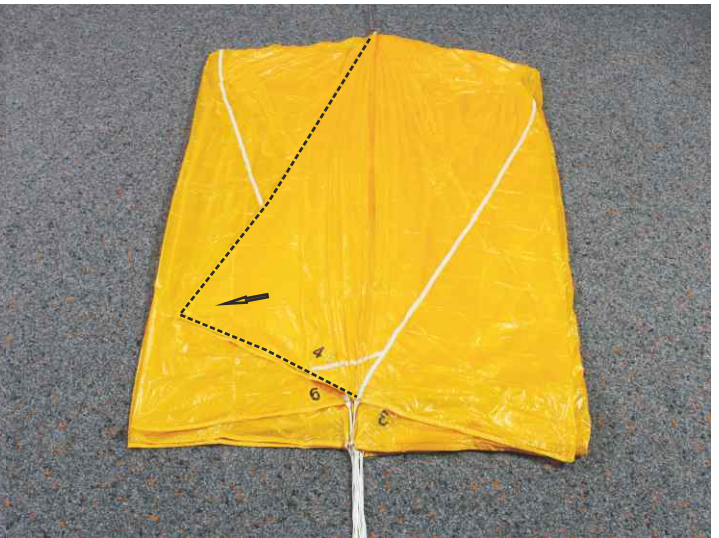
16. Arrange panel 4 (Ultra Cross 100/125). Ultra Cross 150: panel 5
