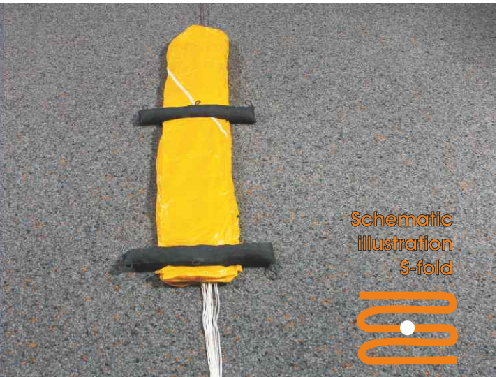
22. Fold left side S-shaped (Step 2).
