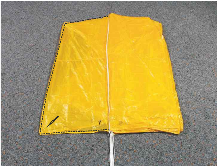
13. Arrange panel 7 (Ultra Cross 100/125). Ultra Cross 150: panel 9
