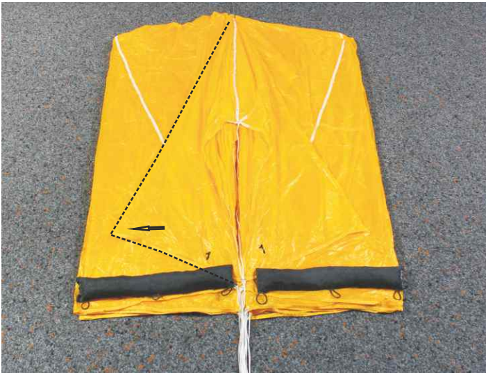
19. Arrange panel 1 (corner panel).
