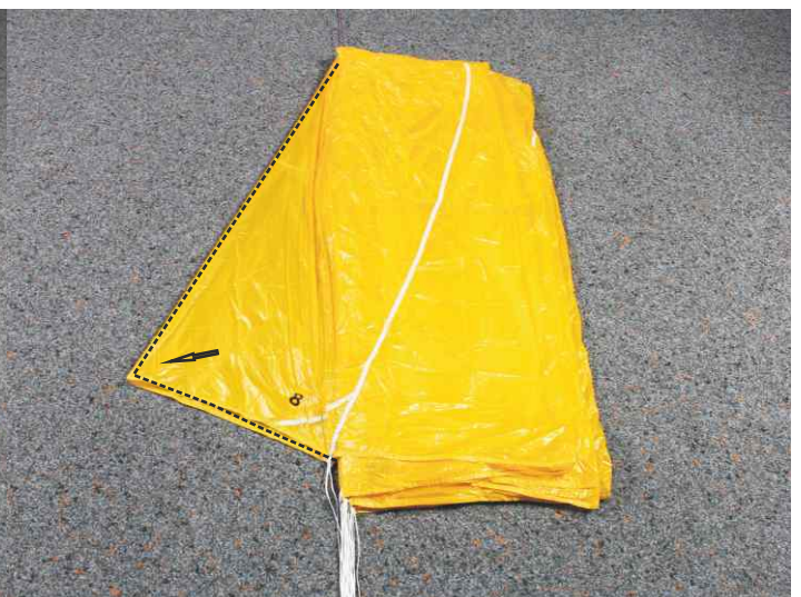
12. Place panel 9 (Ultra Cross 100/125) centered to the the floor and arrange panel 8 to the side. Ultra Cross 150: panel 11/10
