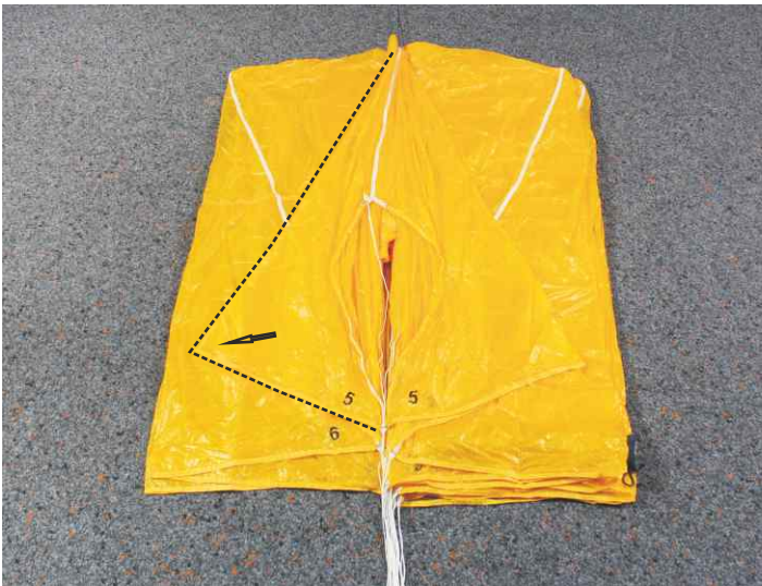
15. Arrange panel 5 (Ultra Cross 100/125) (corner panel). Ultra Cross 150: panel 6
