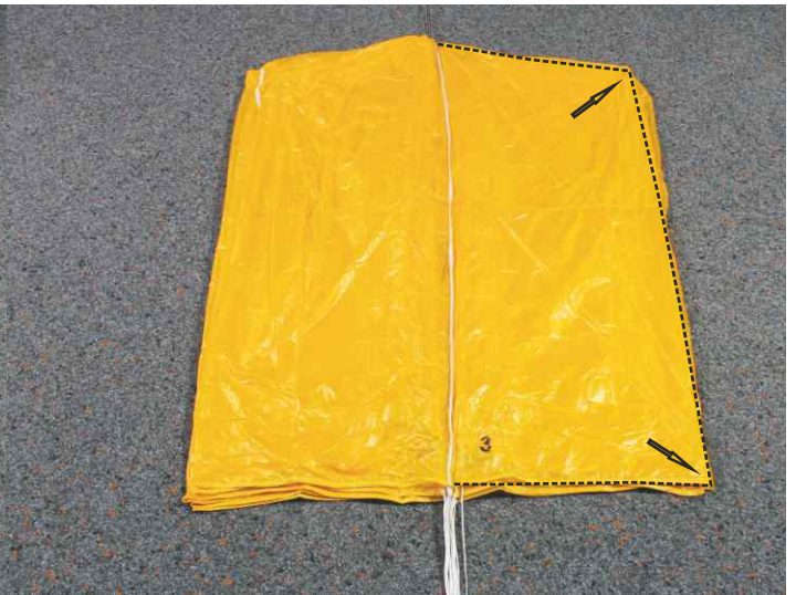
8. Arrange panel 3 (Ultra Cross 100/125). Ultra Cross 150: panels 4,3
