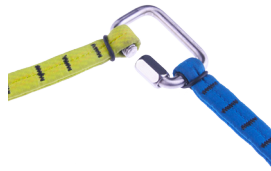
Attach the rescue to the maillon and secure with a rubber band
