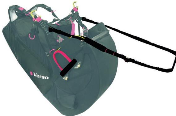
To install the optional quick release footstrap, wrap the webbing of the footstrap around the D-ring. Ensure that the 2 rings line up with each other and that the cord loop is pushed through the rings. Route the long yellow plastic line through the neoprene tunnel, velcro strap at the end of the seat, and the cord loop that is protruding through the footstrap rings. Finally, tuck the plastic line into the neoprene cover of the footstrap.
